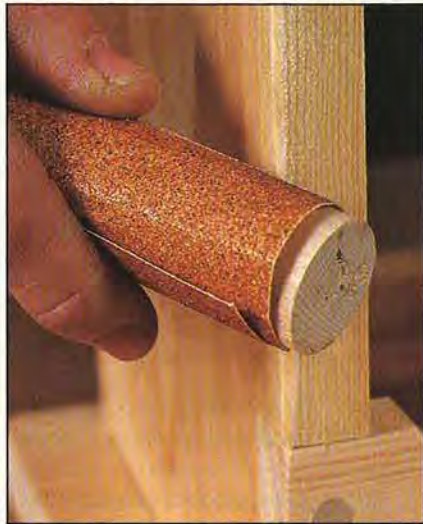
For an edge-rounding tool, wrap 80-grit sandpaper around a 1" dowel.
