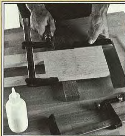
Check that the ends are flush when clamping the front-apron pieces.
