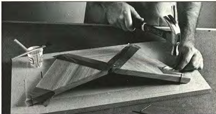
Drive nails into a scrap board around the perimeter of the roof half-section to hold the assembly together until the glue cures.
