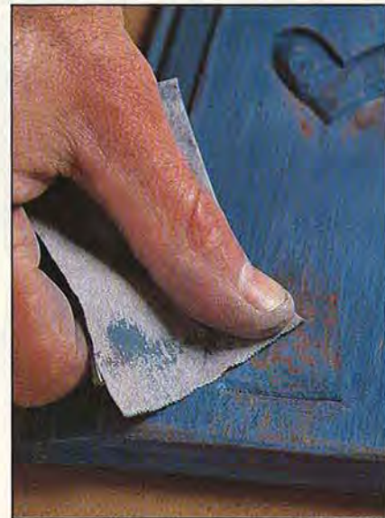
320-grit sandpaper helps you remove the color coat without sanding through the primer.
