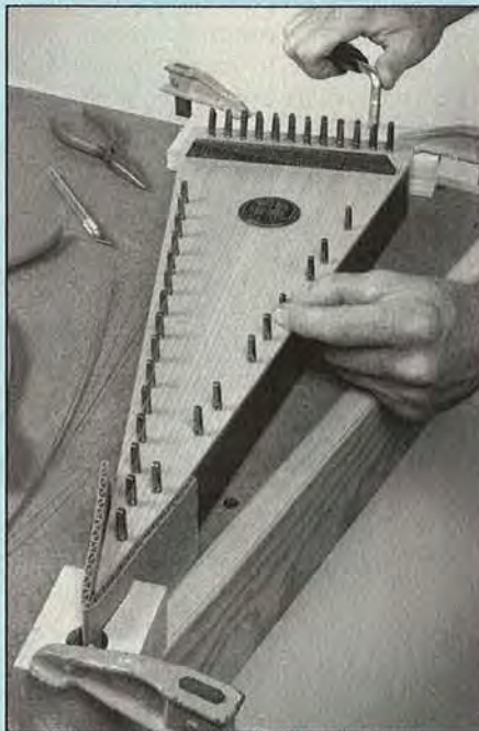
Clamp the psaltery body to your workbench, and tighten the wires between the hitch and tuning pins.
