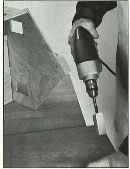
Using the previously drilled hole in the chimney cap as a guide, drill a \frac{1}{4} " hole through the roof.
