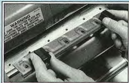
Two magnets safely hold together Makita's blade and holder for attachment to the cutterhead.
