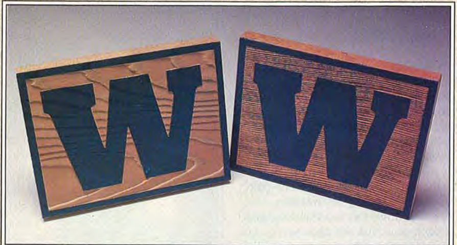
Face- (left) and edge-grain pieces of redwood have different sandblasted looks.
