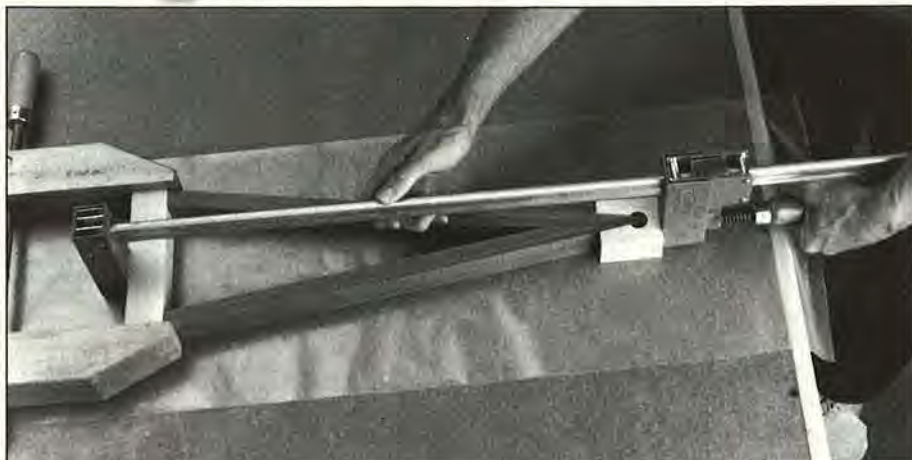
With the top and bottom surfaces flush, epoxy and clamp the walnut side rails to the maple pin block.
