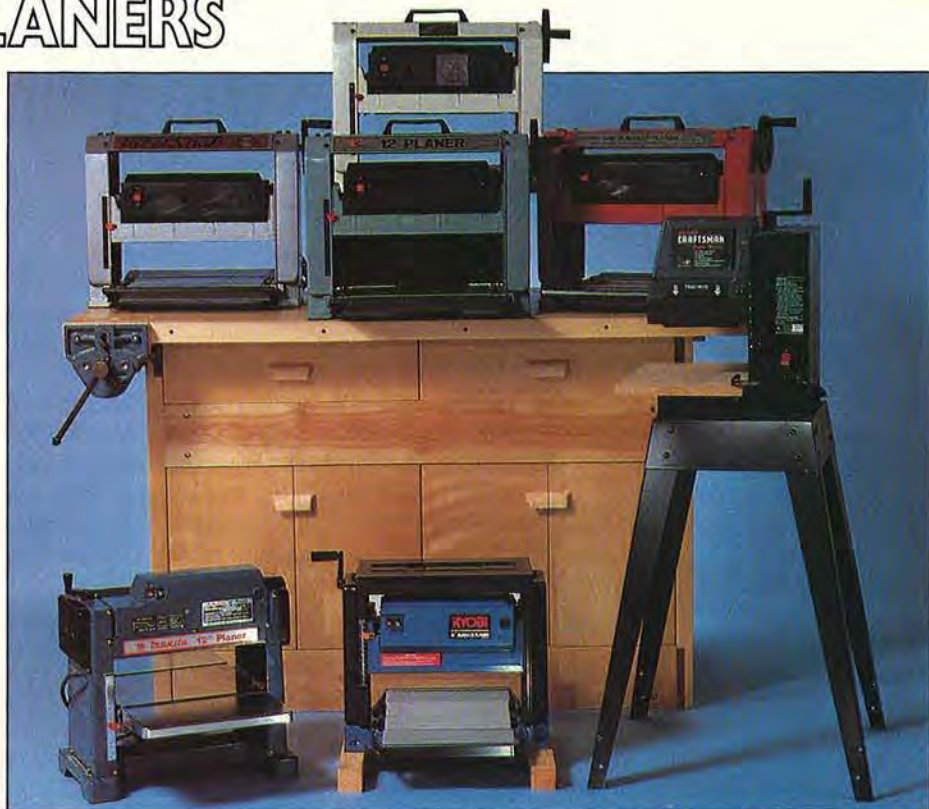
We tested these portable thicknessers: front row from left: Makita 2012 (capable of a 12"-wide cut), Ryobi AP-10 (10" capacity), and Sears 23381 (12" capacity in two passes); and four nearly identical Taiwanese-made 12" thickness planers on the benchtop from left: Total Shop, Transpower, Jet (at top), and Penn State.
