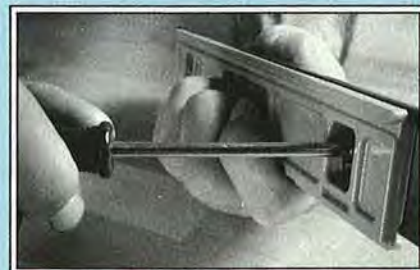
A plastic jig and Phillips screwdriver make easy work of aligning Ryobi's blade and holder.
