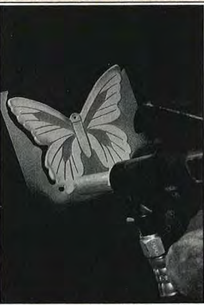
With a sandblaster, you can cut intricate shapes precisely and quickly.
