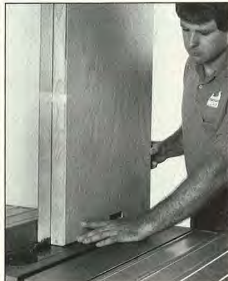
Position the tablesaw fence, raise the blade, and cut one edge at a time to saw the storage case in two.
