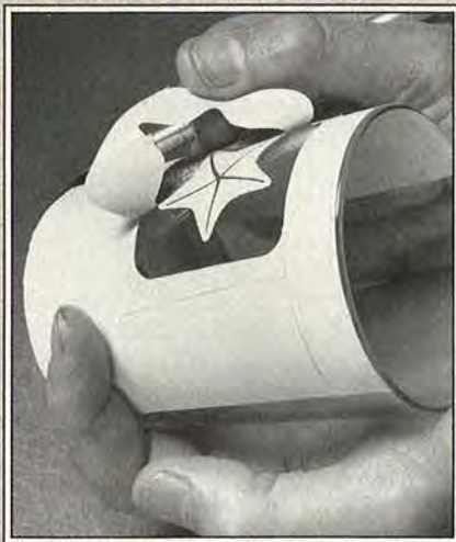
After lifting the edge of the resist with an X-acto knife, peel it away to expose the areas that receive sandblasting.
