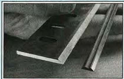
Makita's throwaway blade, right, has two edges versus the one resharpenable edge on Ryobi's blade.
