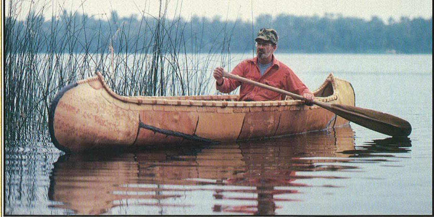
Its seams sealed with roofing cement and bark shrunken tight to the ribs, the canoe takes a maiden voyage.
