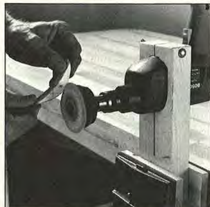
Sand slight round-overs on the front face of each pattern piece.
