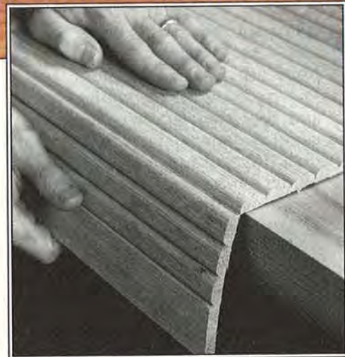
Use the corner of a tabletop to break the glue between the slats.
