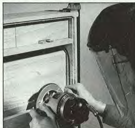
Clamp the upper unit in position on the desk base, and rout a rabbet to house the plywood back.
