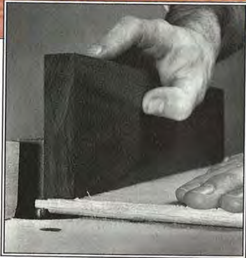
Hold down the tambour firmly when routing the rabbet.
