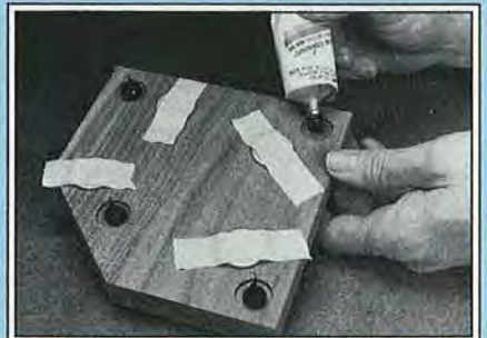
Form nonskid feet by placing silicone sealant in each counterbore.
