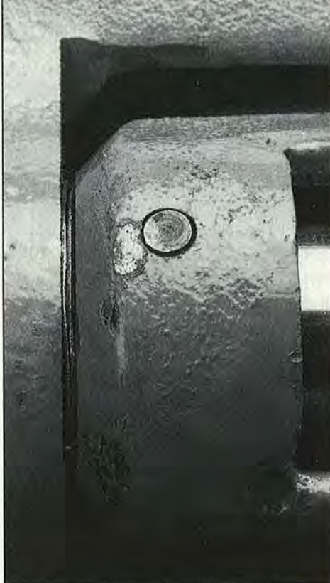
We discovered a tight yoke/motor bracket assembly ( left ) on the Delta 34-763. The similar assembly on the Jet CTAS-10-1 had a gap as shown at right .
