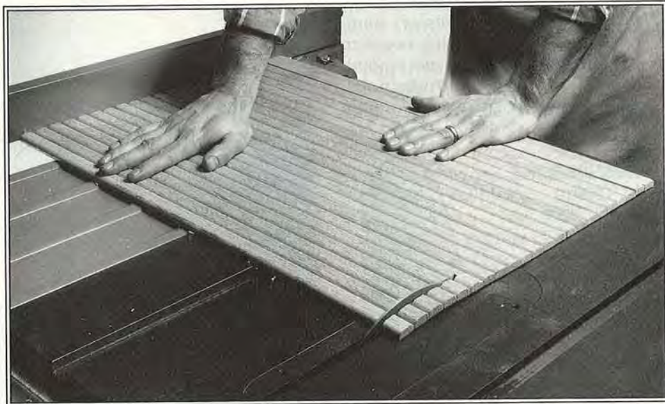
Trim the curtain with your tablesaw and stand to the side of the blade in case it ejects small slat pieces.
