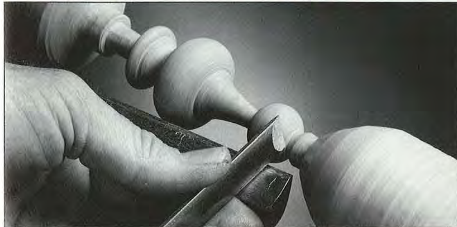
Shape the finial with a skew chisel.
