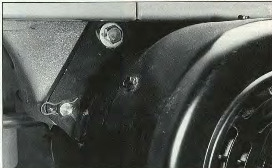
Thanks to the universal bracket shown at right on the General 350-1, you can replace its motor with any motor. That's not that case with the welded-flange bracket on the Delta 34-763, above , that accepts only Delta motors.
