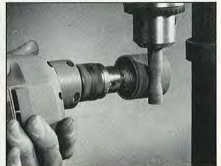
With a portable drill and drill press running, sand the handles to shape.
