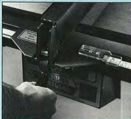
The fence on the Foley-Belsaw 490 helps you make fast and accurate rip cuts.
