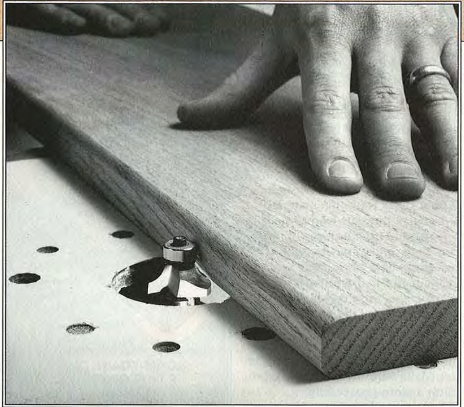
Rout slowly to avoid splintering as you shape the tambour slat.
