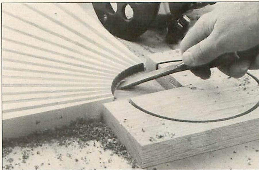
After routing the excess material, clean the surface between the routed area and circle-cutter groove with a sharp chisel.
