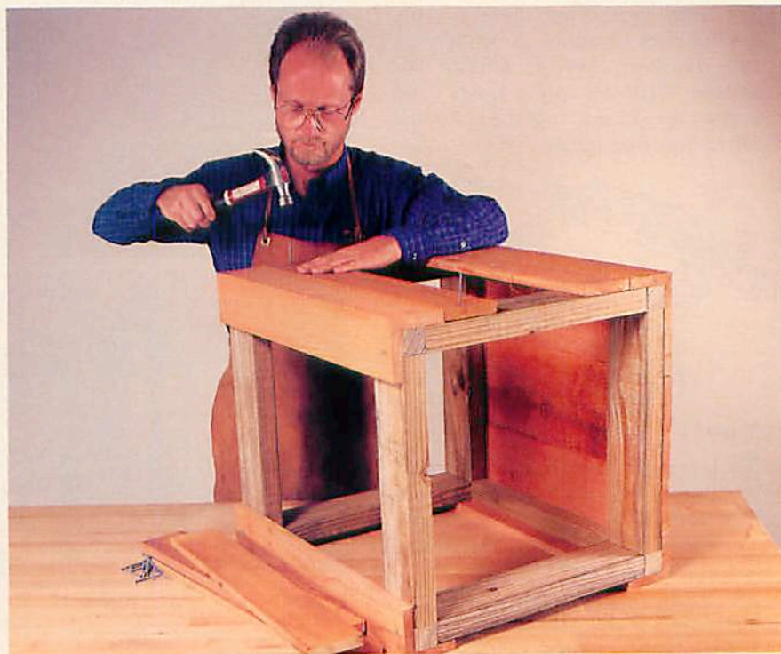
After assembling the skeleton frame, nail the siding pieces in place by starting at the outside and working in. Plane the center piece to fit.
