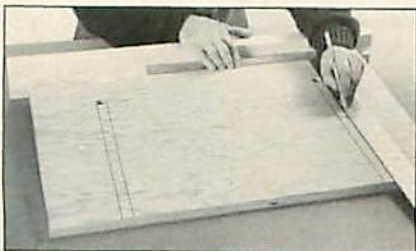
Mark lines on the adjustable support, perpendicular to the beam, on each side of the holes.
