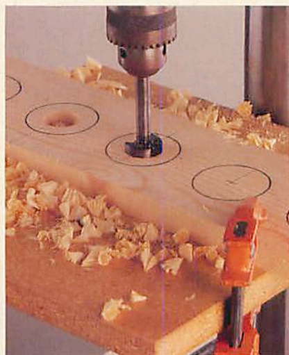
Mark the wheel center point locations on the pine, and drill holes \frac{1}{2} " deep for each outside wheel.
