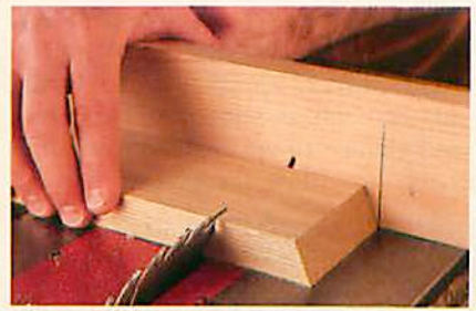
For bowls with horizontal grain, make your first bevel-cut, mark a cutoff line on the auxiliary fence, flip the board over, and make the second cut.
