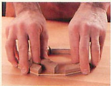
Dry-clip the test staves to check for angle accuracy.
