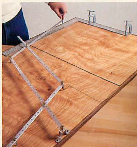
Follow the outline of the copy-area rectangle with the tracing point to mark the 4:1 ratio rectangle on the drawing board. Darken lines with a felt-tip marker.
