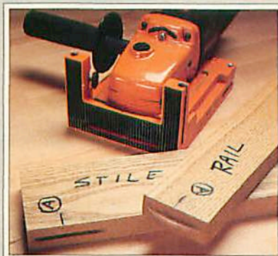
Cutting narrow rails is no problem with the ribbed Kaiser fence.
