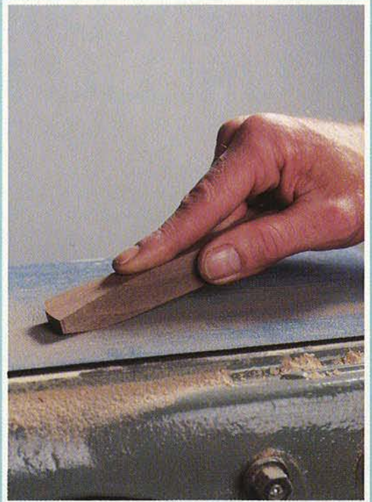
We found our stationary belt sander an excellent tool for quickly sculpting larger parts. You also can shape the parts on a disk sander or drum sander. Shape smaller parts by hand sanding.
