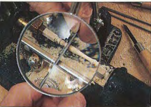
For turning a table leg, Noral employs magnification. He uses a jeweler's file to shape the 1/8" basswood stock held by the adjustable "Yankee" chuck.
