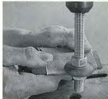
Sanding the walnut disk to shape on a drill press.
