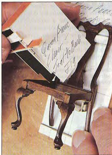
To hold the Queen Anne chair in the correct position for gluing its curved frame, Noral made a jig from illustration board.
