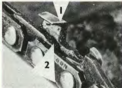
Dull cutters reflect light from their leading edge (arrow 1). Deep filing damages chain straps (arrow 2).
