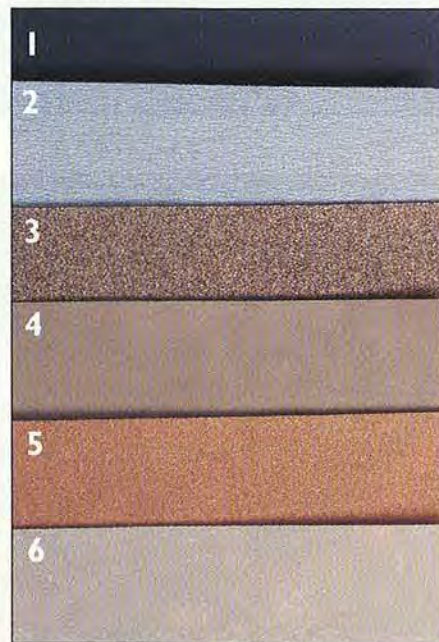
Abrasive minerals by color: 1. silicon carbide, 2. aluminum oxide (coated with zinc stearate), 3. aluminum oxide (coarse) 4. aluminum oxide (fine), 5. garnet, 6. flint.
