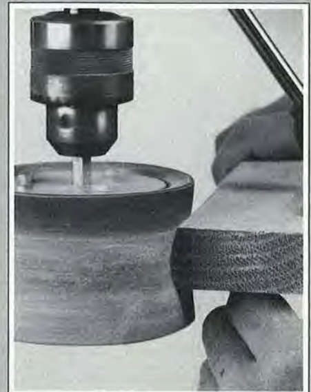
Inflatable drum sanders fit portable drills, drill presses, and lathes. You inflate them with an air pump.
