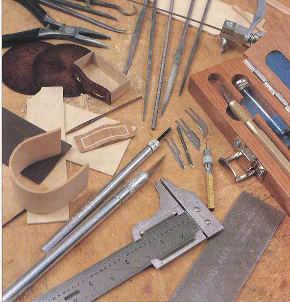
A shoebox holds all the tools you need for building miniature furniture. Jeweler's files double as lathe tools. An X-acto knife becomes your table saw. Other tools Noral has collected from various sources fill the bill for tiny tasks.
