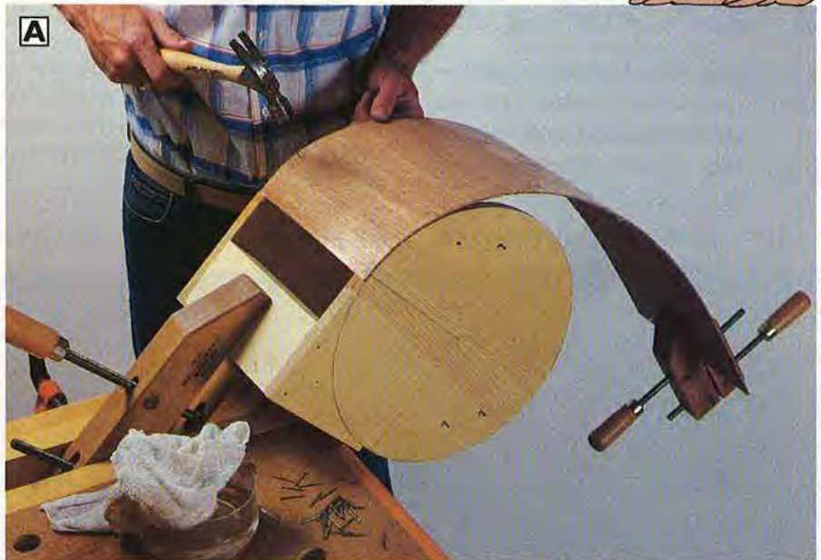
Moisten the plywood with warm water, start it in the cut notch, and then glue and nail it as you wrap it around the stroller sides.
