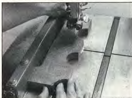
To complete the curved cutouts, band saw between the drilled holes using the saw's fence as a guide.
