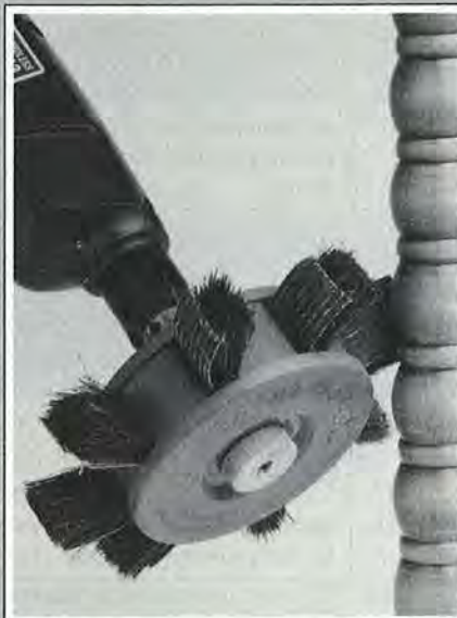
Flapper-type sanders fit portable drills. The one shown here is the Sand-O-Flex from Merit Abrasives.
