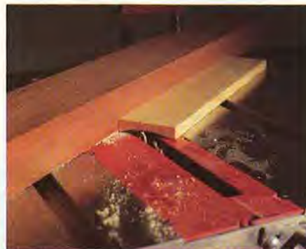
Use the table saw and an angled fence to cove the dozer blade.
