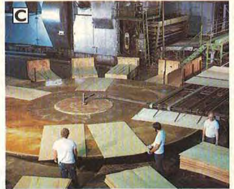
Fresh from the drying oven, plies get sorted on the roundtable.
