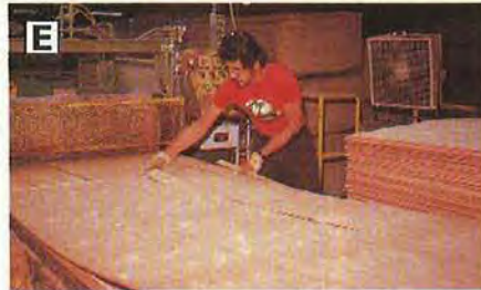
After checking for voids on cross plies, a worker lays the back ply.
