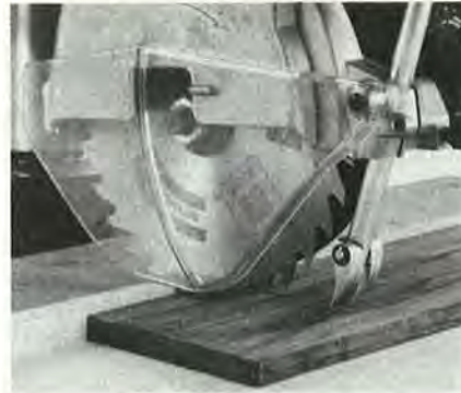
Unlike thin steel guards on most saws, plastic lower blade guard on Ryobi RA 200 doesn't catch in saw kerfs cut in the fence. Anti-kickback pawl (in front of blade) helps prevent kickback.
