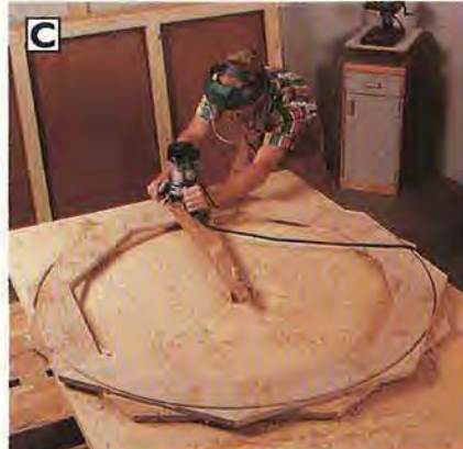
C Mount the trammel and rout the laminated-oak band to shape.
