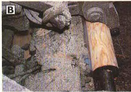
The lathe blade reduces log after log to mere fence posts.
