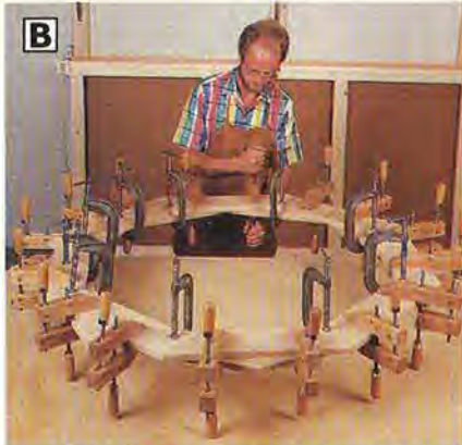
B Apply glue, then align and clamp the two oak bands together.
