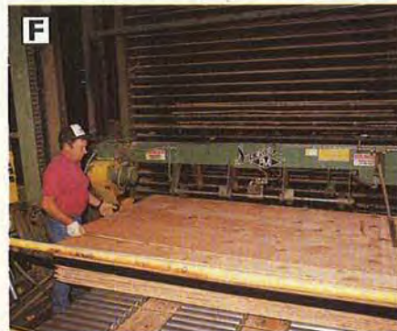
The two-story press bakes and squeezes the laid-up plies.
