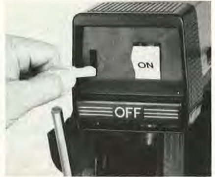
Keyed switch lock on 10" DeWalt 7749 prevents unauthorized use of saw. Delta, Ryobi, and Sears also offer this feature. Large, slap-type OFF switch allows you to turn off the saw quickly in an emergency.
