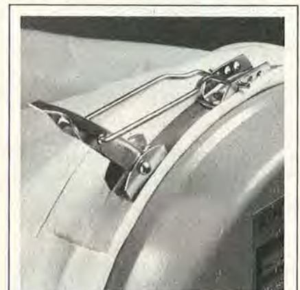
The Kraemer uses a wide steel band clamp with a quick-release to fasten the filter bag to the blower outlet.
