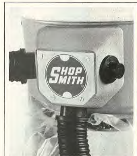
The Shopsmith collector uses three 2½"-diameter hoses to fit Shopsmith woodworking machines. In this photo, we've connected two of them to the collector. To add a third, you remove the plastic plug at right. Standard features include an adapter for a 4" hose, and attachments.
