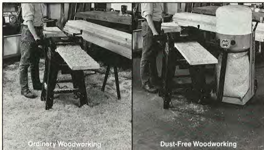
Unretouched photos after planing 100 square feet of surface area.
