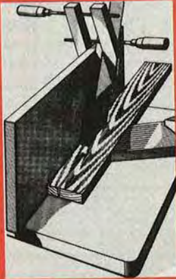
Use this setup for ripping long, thin stock.
