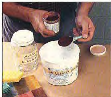
Measure and mix. A tablespoon of aniline powder makes a quart of dye.
