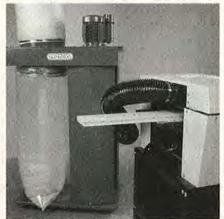
A "plane" advantage. Thickness planers and jointers spit out more heavy chips and wood shavings than any other woodworking machine. The right-size dust collector will bag 95% of the stuff. Here we have the Inca collector connected to our 13" Foley-Belsaw planer.
