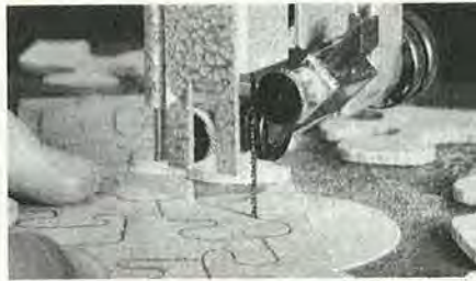
Above: Inca solved the puzzle of fitting a \frac{1}{16} "-wide blade in a band saw. A special grooved roller guide replaces the standard roller bearing. Right: The Royobi BS-50N comes equipped with a 2"-wide blade to accurately resaw boards up to 7" wide; takes blades down to \frac{1}{4} ".
