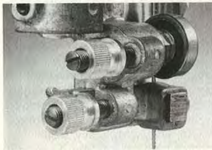
Above: Microadjustments on Delta 14" saw provide precision control on roller guides and guide-assembly carriage.
