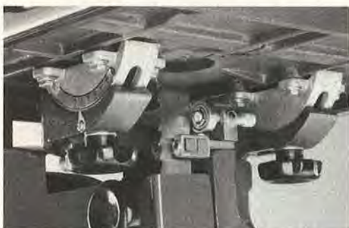
Sturdy trunnions provide solid support for the heavy cast-iron table on the Grizzly 18" saw. Tilting this saw's table is easier than you may think.
