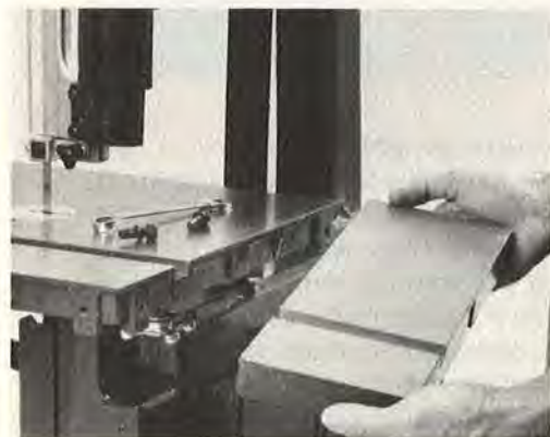
Small table extension attaches to front or either side of table on AMT 14" saw. This saw also has optional riser block to extend cutting height to 12".
