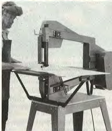
At 24½", the Woodmaster Model 500 has the deepest throat capacity of all saws we reviewed. Above , we're using it to scallop the edge of a 2'-wide panel. Optional table extenders made it a one-man job.
