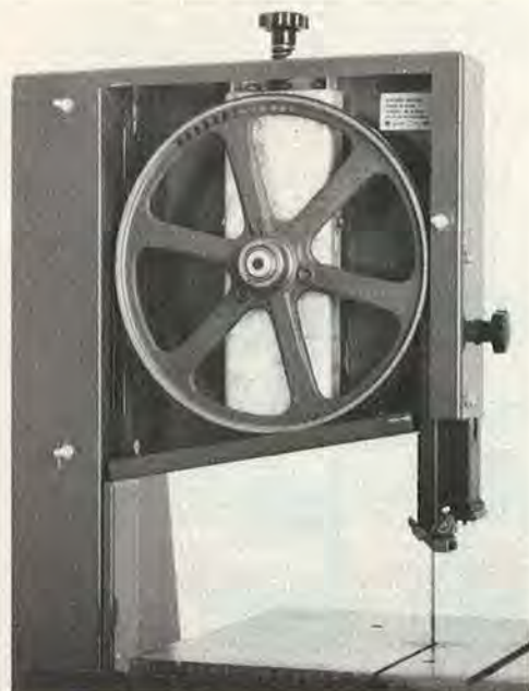
Mini Max precision-balances their cast-iron band saw wheels by drilling holes in the rim. We found this saw runs smoother than all the others we tried.
