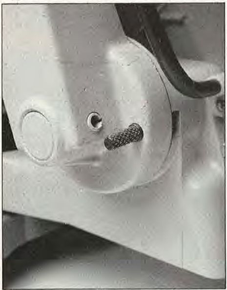
The surest motor hold-down for storage or transport is the reliable pushpin, shown on this Delta 34-010.
