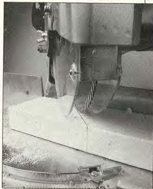
The rear-hinged guard on the Hitachi C 10FA lifts out of the line of vision before the blade makes contact.
