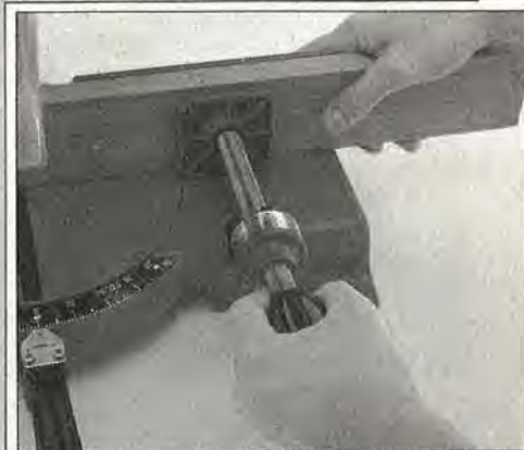
Makita miter saws feature this handy-to-use quick-release vise.
