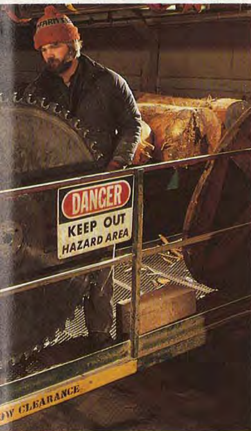
Above. Replacing the 56" blade requires two men. Tim Hohmann, left, the fix-it-all millwright, helps Brad Olsen, a sawyer, move the blade to Line No. 2.
