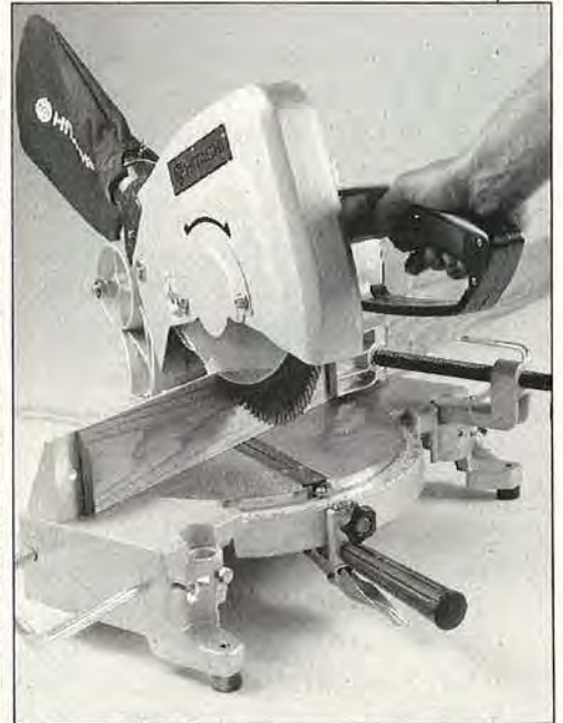
Note the cut-through plastic slot of this Hitachi C 10 FA. This design feature ensures you a tight blade fit.
