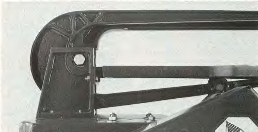
The RBI Eagle C-arm has a centered pivot point above the table which causes the blade to tip slightly forward at the bottom of the stroke.
