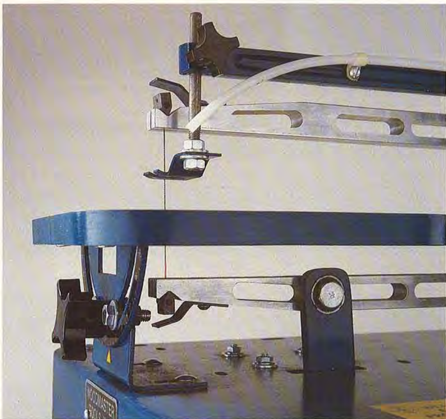
Long tie rod with motor mounted below base in Woodmaster (note also the two-way tilt table)
