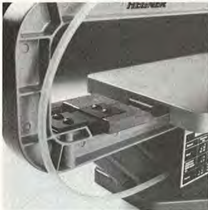
The short-stroke Hegner Hobbymax uses a spring steel plate as a pivot point for the C-style arms.
