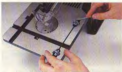
Sears built-in blade clamp holders for precise distancing
