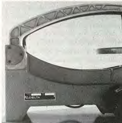
The Delta C-arm saw has an off-center pivot point at table height to keep the blade vertical at the bottom of the stroke.
