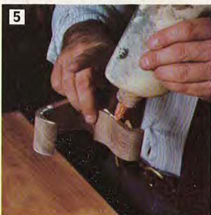
5 Gluing and assembly. With yellow glue, Richard readies a compartment for its front and back pieces.
