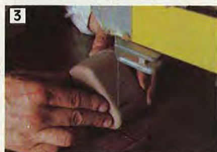
3 Making the compartments. Slicing off the core's front and back, then sawing out its center, creates a box.
