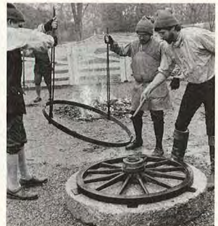
The iron tire, after heating in the fire, is about to be dropped over the wheel. An old millstone serves as the tiring platform.
