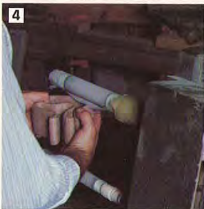
4 Contour-sanding. Sandpaper-covered spindles of varying sizes were shop-built to conform to different shapes.
