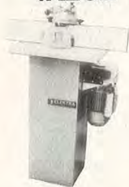
TF100M 3 speed shaper, 3 HP, $985.00, CAP 6" x 4 1/4" stroke
