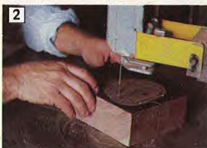
2 Band sawing the box. A \frac{1}{8} " blade follows the outline contours as the box is cut from the stock.
