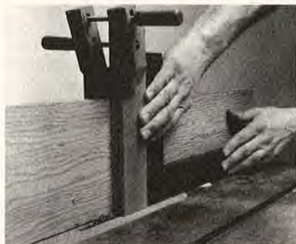
A follow block adds stability and prevents chipout of the workpiece
