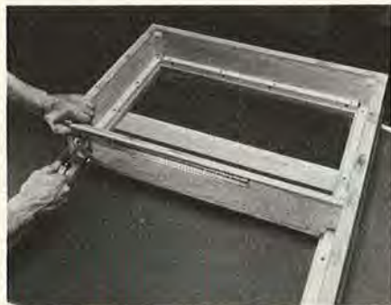
Mount the drawer slides flush with the bottom of the guide rails
