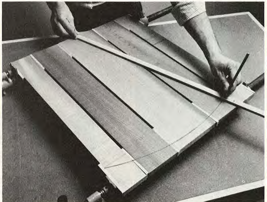
Mark the seat radius with a trammel of scrap wood
