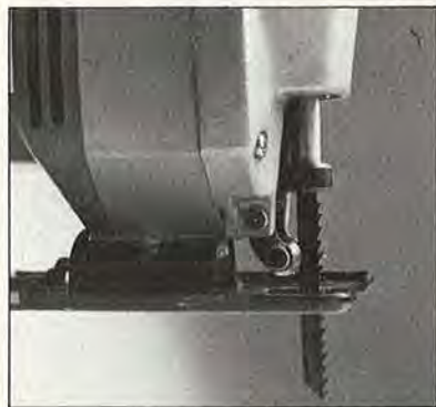
The roller guide at the back of this Ryobi and other models relieves the stress on the ram shaft and keeps the blade running true.
