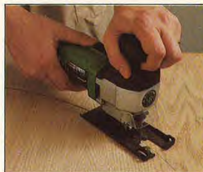
The barrel and knob grip on this Hitachi jigsaw allows excellent control.
