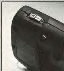
Some electronic saws like this Metabo have the speed control dial near the front for convenience while cutting.
