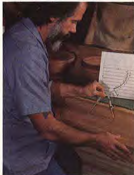
Step 1: From dimensions drawn on paper, Bob transcribes the cutting lines on stock with a compass.
