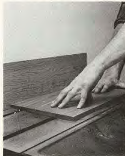
The panel-raising sequence begins when you make shoulder cuts along the edges of the glued-up panel
