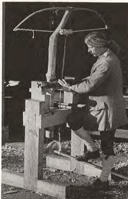
The foot-operated spring-pole lathe, a European invention, commonly runs at about 900 r.p.m.
