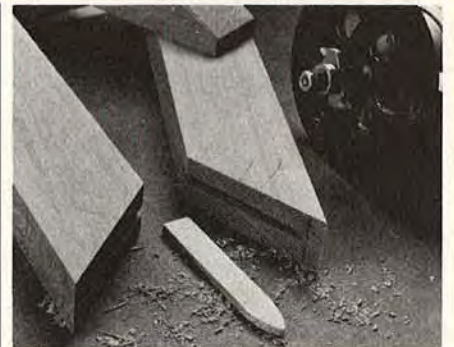
Tenon spline joinery fortifies an otherwise weak miter joint
