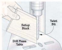
1] Hold an angled setup block against a long twist bit to set the angle of the drill press table.
