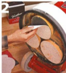
SWITCH DISCS OFTEN To speed up the sanding process, change discs as soon as they clog with the old finish.
