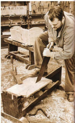
A low bench positions boards at the right height for ripping. Thick stock and dovetail joints make the bench sturdy, while wide feet and a shelf loaded with bricks keep it stable.
