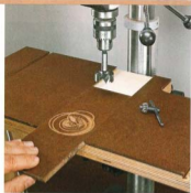
Mating bevels keep this replaceable insert securely on the drill press table.
