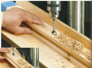
This drilling jig ensures accurate, evenly spaced holes thanks to its built-in index pin. The pin also prevents the angled strips from sliding as you drill.
