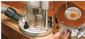
Triton's dust-collection port (left) is built into the base of the router, and two see-through shields allow little space for dust to exit anywhere else. The DeWalt dust port (right) has to be mounted from underneath the router base.
