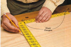
Mount both stair gauges to one leg of a framing square to create a super-size try square for marking wide panels.
