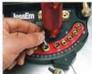
1] A large primary pin locks the miter gauge at 5° increments between 0° and 45° in both directions.
