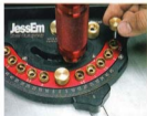
2] Use the smaller secondary pin to make half-degree adjustments between the 5° detents.
