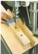
To drill evenly spaced, angled holes in the keeper strips for the balusters, I used this drill press jig (see page 88).
