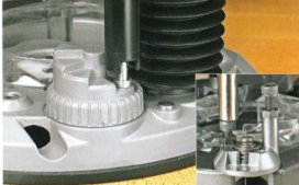
Five fixed positions on the Bosch turret (above) make it easier to rout a series of progressively deeper passes than turrets with just three adjustable positions (inset).
