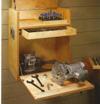
By mounting it on a wall, this job box becomes a nice shop cabinet, complete with a drop-down work surface.
