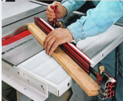
A telescoping fence, adjustable scale, and a flip-stop allow for accurate, repeatable cuts on workpieces up to 36" long.
