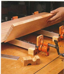
These cradles hold aluminum rails that raise the glued-up panel off the clamps. This centers the clamping pressure on the thickness of the stock, so you end up with a flat panel.
