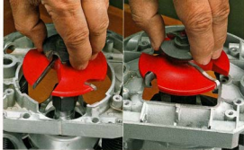
Bosch's large base opening (left) easily accommodates a 3½" panel-raising bit. The much smaller opening on the Freud (right) makes using bits this large difficult.
