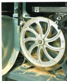
A band saw blade pulls a lot of dust into the lower saw cabinet.
