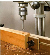
Adding a fence and stop blocks enhances the precision and accuracy of the drill press table.
