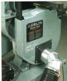
A 4" port on the lower door catches dust that gets pulled into the cabinet.
