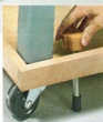
Adjustable "feet" raise the base off the casters to stabilize the tool.
