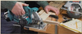
▲ The crosscut test was performed twice with each saw to ensure accurate results and allow for differences in stock. A crosscut sled guaranteed uniform cuts.
