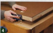
▲ Finally, use a hand plane to trim the edges of the torsion panel. A few quick strokes is all it takes to make the exposed edges of the core pieces flush with the skins.
