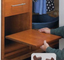
▲ A groove cut in the sides of the adjustable shelves allow them to slide onto low-profile supports (shown above). The supports are available from Rockler (800-279-4441).
