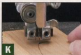
▲ The Delta's guidepost provides a clear sight line — even with the guides very close to the workpiece.
