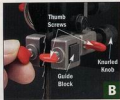
▲ Thumbscrews on Ridgid's guide system make it completely tool-less. A knurled knob positions the guides.
