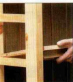
▲ Notches on the ends of the shelves fit around the corner posts to keep the shelves from moving front to back.
