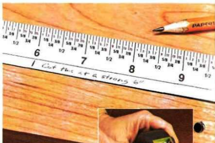
▲ The Story Pole tape is designed to be written on with a pencil. It has standard measurements and room at the bottom for writing notes.
