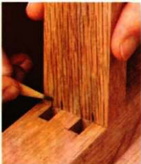
▲ The completed mortises provide an accurate guide for laying out the tenons on the ends of the rails.
