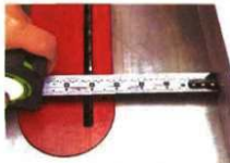
▲ The Lefty/Righty tape features a measuring scale along both edges of the blade, so the markings are easy to read whether you're measuring from the left or the right. This feature comes in particularly handy when checking the distance from the rip fence to your saw blade.
