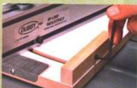
Positive 90° Setting. An adjustable stop makes it easy to quickly return the fence to a 90° setting for right angle crosscuts. You'll find this feature on all the miter sleds.
