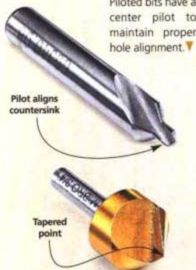
▲ Non-piloted bits have no center pilot and require the drilling of a pilot hole first.
