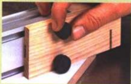
Adjustable Backer Board. A replaceable wood extension on the end of the fence of this miter sled allows you to back up your workpiece completely when making a cut.
