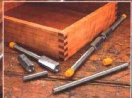
▲ For smaller drawers, you can use a pair of coupling nuts. Several different lengths of threaded rod will make it easy to square any size drawer.
