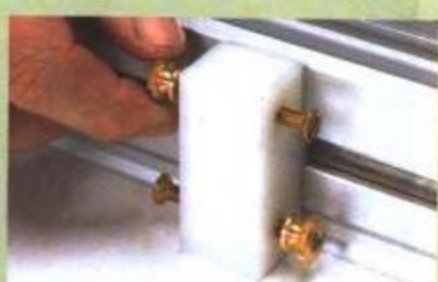
Adjustable Stop. An adjustable stop on the fence allows you to cut multiple pieces to the same length. This stop is reversible, giving you two settings.
