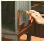
Dark Basecoat. After waxing, the first of two coats of "soldier blue" milk paint were applied. A cheap foam brush works fine and I made a quick job of it.
