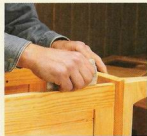
Sandpaper. The first step is to add a little wear and tear. Use some coarse sandpaper to knock off the sharp edges and add some "age" in the right spots.
