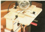
▲ This simple mortising jig makes it easy to rout mortises on the end of a workpiece or on its edge. To build one, turn to page 18.
