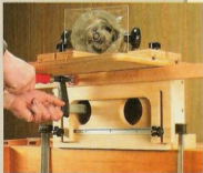
▲ The horizontal fence supports a long workpiece when cutting mortises along the edge.
