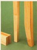
Glued-up Blank. A three-piece glueup creates the right thickness, but also a lot of color and grain variation.
