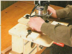
▲ Clamp the workpiece to the jig, then position the stops. That's all it takes to set up this jig for routing mortises in just about any workpiece.
