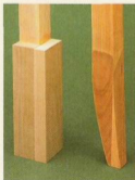
Add-on. Gluing scraps onto the bottom of a square blank to form a foot leaves too many glue lines.
