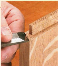
▲ A sharp chisel makes paring away the step easy. Just take a shallow cut and the wood will "curl" away.
