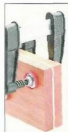
Bracket feet look like they were cut from thick blocks of wood, but these blanks were made with two pieces of ¾"-thick stock.
