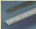
Etched blade. A satin-chrome finish and finely-etched markings make the lower rule in this photo easier to read than the die-stamped rule above.
