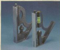
Cast iron. Better squares usually have a head made of fine-grain cast iron (left). The head on the right is a rougher version made of die-cast metal.
