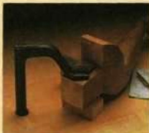
Holdfast. This simple holdfast is a traditional clamp that can be used to secure a workpiece to the top of your workbench.
