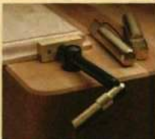
Bench Dogs. These bench dogs (right) and Wonder Dog (left) are modern tools for making your workbench more useful.
