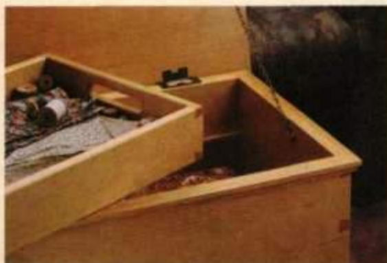
Sliding Tray. Like the case, the sliding tray inside the chest is joined with hand-cut dovetails. This tray sits on simple supports glued into the front and back of the case.
