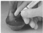
Touching up the color. There are a number of solutions for applying color to a scratch or a dent. This touch-up marker is a quick way to add both stain and finish.
