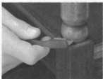
Cleaning tight spots. When you've got to clean turned spindles and intricate carvings, a toothbrush is handy for getting into those hard-to-reach places.
