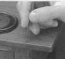
Restoring the color. A little stain will hide nicks and scratches. And it doesn't have to match perfectly either. The goal is to minimize the contrast in color.
