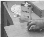
Removing the grime. The first step with any project is to clean it with naphtha and a soft rag. This solvent dries quickly and won't damage the wood.
