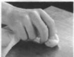
Applying a temporary fix. Paste wax will raise the sheen of a finish and can hide scratches. To apply a thin, even coat to a large area, place a ball of wax in a cloth.
