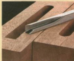
A Square ends. Like driving a square peg in a round hole, this corner chisel squares up the rounded ends of mortise.
