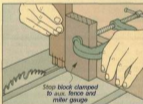
Inside cheeks. The inside cheeks of the tenons are cut with the workpiece standing on end. A stop block clamped to the auxiliary fence helps support the workpiece.
