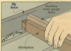
Outside cheeks. All cuts for the twin tenons can be made on the table saw. An auxiliary fence on the miter gauge prevents chipping on the back side of the cut.
