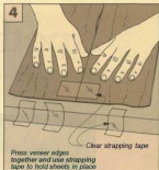
Joining the pieces. As the veneer pieces are butted together, use clear strapping tape to "clamp" them until the glue dries.
