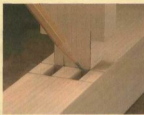
Mark tenons from mortises. The mortises on the leg can be used to quickly indicate the position of the tenons on the rail.
