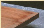
Low spots. After wet-sanding, high spots in the finish show up as dull areas. Sand until the low shiny areas become dull too.
