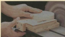
A This jig allows you to accurately sand a wide variety of different sized circles. And if you need several pieces the same size, the built-in stop makes it easy.
