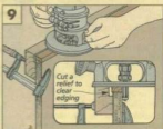
Flush Trim Bit. The quickest way to trim a lot of edging is with a flush trim bit. Clamp a board to one side for more router support.
