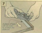
Block Plane. To help prevent tearout, hold the block plane at an angle to make a shearing cut along the edging.
