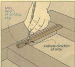
Measure Direct. When fitting small strips of molding, it's always more accurate to take a direct measurement than it is to use a tape.
