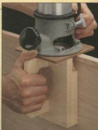
A The handle on the jig holds the router steady while trimming the edging flush along the length of the plywood.
