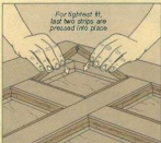
Press Fit. If the last strip of molding is cut to fit perfectly, it may be difficult to insert. Instead, insert the last two at the same time.
