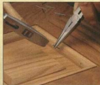
Panel. After the frame has been glued up, the panels are secured with strips of molding. And unlike traditional panels, these panels will keep a tight seal.
