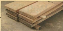
Direct from the lumberyard, dimension lumber is usually wet. But it won't take long to dry in a home shop. For good air circulation, "stick" the boards so they're off the ground and not touching.
