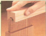
To "dress up" the through tenons, the ends are chamfered. A simple sanding block helps keep the chamfers consistent.
