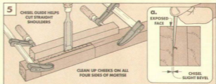
Complete the mortise by chiseling the sides of the mortise smooth and flat. Use the guide block to keep the chisel straight
