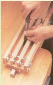
After roughing out the mortise with a drill press (left photo, above), attach the jig to guide a chisel for cleaning up the mortise (right).
