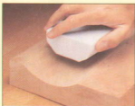
A piece of Styrofoam insulation board can be used to sand an irregular shape. First cut the sanding block to rough shape.
