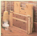
To store or move the workbench, just release the draw catches. Then, lift off the top and fold in the legs.
