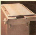
With bench dogs, the clamping capacity of the top is increased from 7" to 17". Big enough for a small panel.
