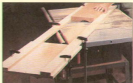
It's easier to cut a cove on a long workpiece with a pair of guides. And a platform (with a support leg) clamped between the guides keeps the piece from tipping down.
