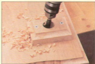
A rectangular block strengthens each leg joint. First, an angled hole is drilled on the drill press. This guides an electric drill that completes the mortise for the leg.
