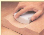
Now peel the sandpaper from the workpiece and stick a fresh piece of sandpaper on the block. Then sand the workpiece.
