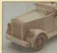
The engine compartment is shaped with two tapers. First the sides, then the top.
