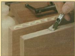
A strong joint requires a thin, consistent layer of glue. For a good bond, apply it to both edges and spread it out with a brush.
