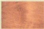
Even with a stain controller, maple can turn out blotchy. The key to minimizing blotchiness is wood selection and sanding.
