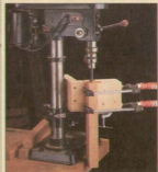
To use the holding jig on a bench-top drill press, first swivel the head over the edge of the bench. Then set up as described at left.
