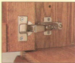
This concealed hinge has two parts. The "cupped" part fits in a hole in the door. Then a mounting plate is screwed to the cabinet.
