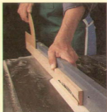
A zero-clearance insert prevents the narrow edge of a workpiece from tipping into the table saw opening. A push stick keeps your hand away from the spinning blade.
