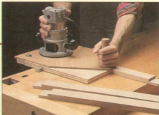
When routing half laps on a narrow workpiece, clamp a scrap of plywood on the outfeed
