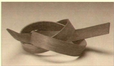
Here's an example of how tight a thin, straight-grained strip of wood can be bent. This 1/2"-thick walnut strip was soaked overnight in tap water and then tied up like a pretzel.
