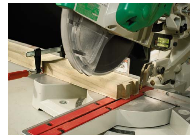
Gang cutting produces multiple identical workpieces.
