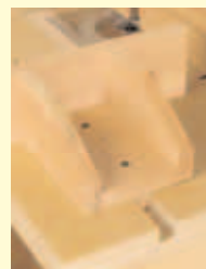
LEFT: The push bar guides stock routing and helps apply even pressure. RIGHT: The fences adjust via elevator bolts and grooves in the top assembly.
