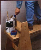
► Mini-Scaffold. By placing the plank on one of the lower stretchers of the sawhorses, you can use it as a platform when you need to reach the high spots.
