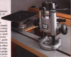
▲ Plunge Base. With an auxiliary plunge base, you can leave the standard base attached to your router table for fast changes between setups.
