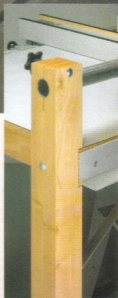
▲ Rigid Support. A beefy hardwood mast and steel conduit anchor the dust cover to the saw table.
