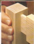
▲ The Result. For tenons with smooth cheeks, crisp shoulders, and a gap-free fit, a dado blade on the table saw is the ticket.
