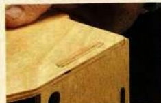
▲ File to Fit. To get the tabs to fit the slots, I used a file to round over the ends. Aim for a slip fit.
