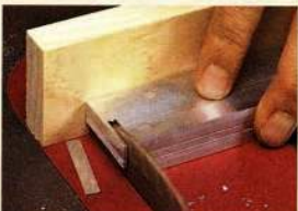
▲ Trim Edges. Use a carbide-tipped blade to trim the blank to final length and square up the sides. Then trim the corner off the end as shown in Figure 2.
