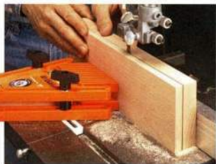
▲ Double-Decker. Feather-Locs can be combined to provide support for tall stock.
