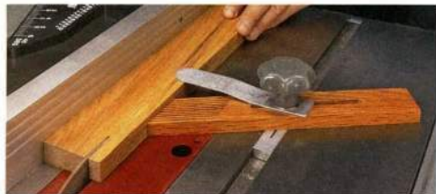
▲ Double-Duty. This hardwood featherboard combines sideways pressure on the workpiece with an aluminum "thumb" to hold the workpiece securely against the saw table.
