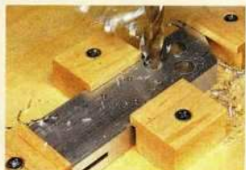
▲ Hole Pattern. Use a \frac{7}{16} "-dia. bit to drill the decorative hole pattern on the handle. A countersink forms the \frac{1}{16} " chamfer around the edge of each hole.
