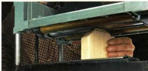
► Align the Cutterhead. An alignment block makes it easy to check that the cutterhead is parallel to the bed.
