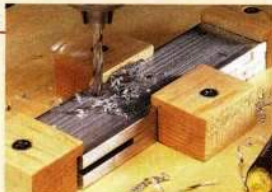
▲ Rivet Holes. Drill \frac{1}{4} "-dia. holes for the rivets, then check the fit. The rivets should slip easily into the hole and completely through to the other side of the blank.
