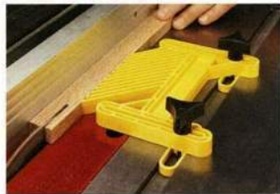
▲ Miter Slot. Securely locked into the miter slot by a pair of “cleats,” this featherboard from Big Horn holds a workpiece tight against the fence.
