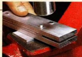
▲ Adding Rivets. A spacer raises the handle so you can "mushroom" the ends of the rivets. Remove the spacer and flip the blank over topeen the other side.
