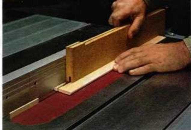
▲ The Right Push. This simple push block gives you complete control when ripping small, thin pieces.
