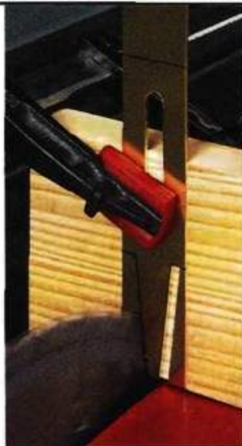
▲ Angled Cuts. Use an auxiliary fence with a shallow dado and clamp to hold the brass in place.
