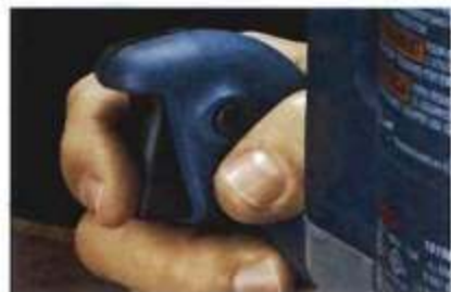
▲ A Handy Switch. You won't have any trouble finding the trigger switch on the handgrip of this plunge router.
