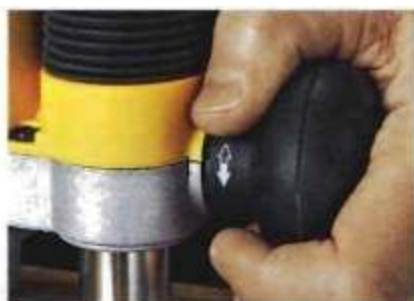
▲ Grip Plunge Lock. Turning the handgrip on this plunge router locks and unlocks the plunge action.
