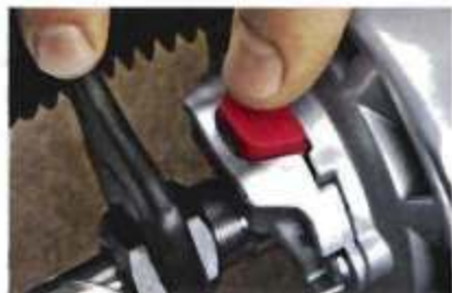
▲ Spindle Lock. Depressing the button locks the spindle so the collet can be tightened or loosened with one wrench.
