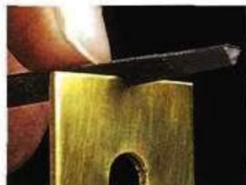
▲ Filing a Notch. A triangular file is ideal for forming the small notch in the end of the brass keys.
