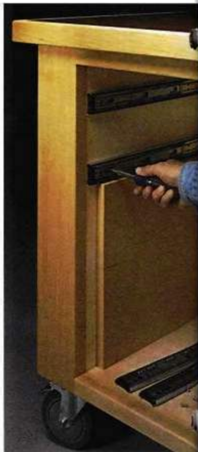
▲ Bottom Slide. A piece of \frac{1}{4} " hardboard positions the slide up off the bottom of the cabinet.
