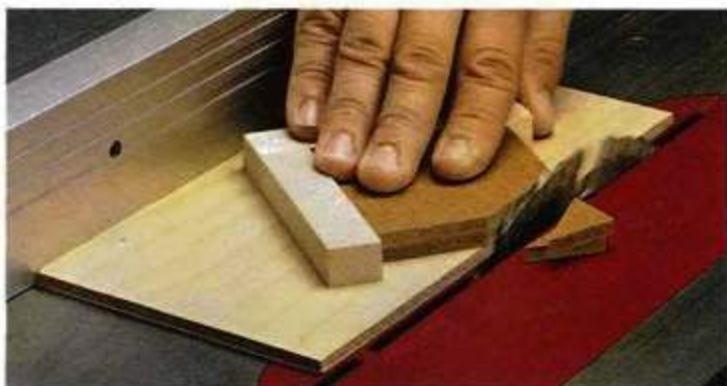
▲ Small Parts on a Sled. Here, a piece of plywood and a couple of cleats position the small pieces and make angled cuts a breeze.
