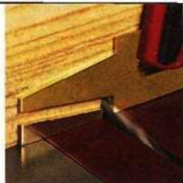
▲ Final Cuts. A zero-clearance insert makes trimming away small pieces easier and safer.
