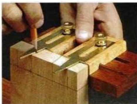
▲ Dovetail Layout. The angled dovetail keys make quick work of spacing and marking the pins of hand-cut dovetail joints.
