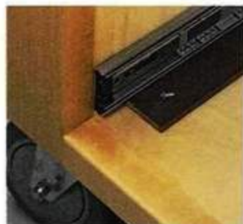
▲ Bottom Slide. A piece of \frac{1}{4} " hardboard positions the slide up off the bottom of the cabinet.
