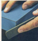
▲ Filing Edges. Downward and outward strokes of a flat mill file make smooth edges.
