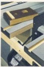
▲ Splitter Insert. Removal of the "pop out" insert makes way for installation of the splitter and blade guard.
