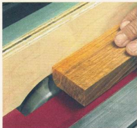
▲ Auxiliary Fence. Burying the knives in an auxiliary rip fence allows you to shape the edge of a board using just a portion of the knife profile.
