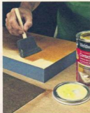
▲ Apply Glue. For best adhesion, apply two coats of contact cement to the laminate and the substrate.
