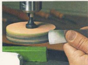
▲ Buffing Wheel. A wheel charged with different grades of abrasive compound can polish the edge of a gouge in no time.
