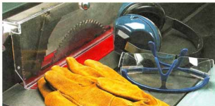
▲ Thinking Safety. The shavings and sharp edges created as you work make eye and ear protection a must. So always wear your safety glasses and ear muffs. In addition to
