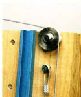
Cable Hook. The cable is attached to the saw base with a hook made from a piece of aluminum angle.
