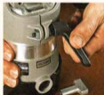
▲ In With the New. An inexpensive solution is to upgrade to an easy-to-grip, lever-type lock.
