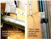
Measuring Tapes. Finally, in the box below, you can see how I added a pair of measuring tapes to set up for accurate cuts.
