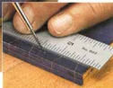
◀ Using Layout Fluid. Coating the surface of the metal makes scribed marks easier to see.
