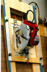
▲ Two-Position Base. The circular saw clips into the base with toggle clamps for ripping and crosscuts.
