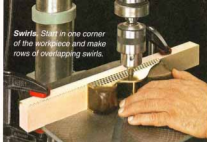
Spacing. Index marks laid out on top of the fence can be used to keep the spacing of the swirl pattern consistent.
