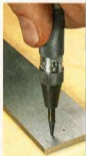
▲ Metal Punch. The spring-loaded punch is easy to use and leaves a handy dimple for starting a drill bit.
