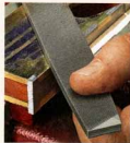
▲ Flat File. When it comes to dressing edges and shaping metal, flat files work quickly.
