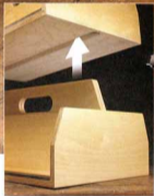
▲ Mating Parts. Stacking the totes is just a matter of slipping one tote over the handle of the one below.
