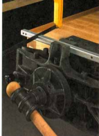
Vertically. Rotating the vise 90° provides a better grip on vertical workpieces.
