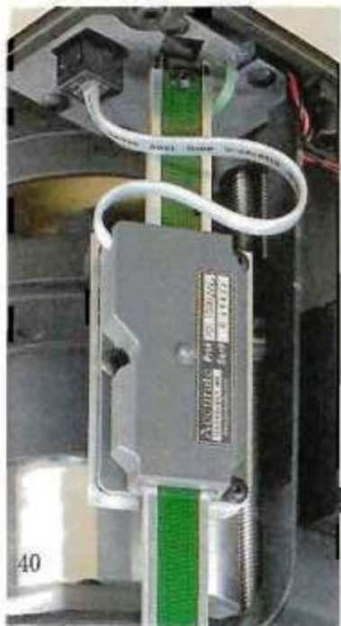
► Guaranteed Accurate to 0.001". The Jointech SmartLift Digital features the Absolute Encoder, from Accurate Technology. The sensor attaches to the carriage, sending precision measurements to the digital display.
