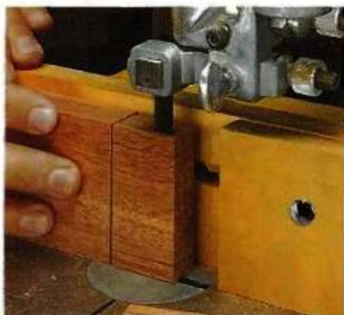
▲ Cutting the Cheeks. This time, carefully cut just to the shoulder line. This leaves a crisp edge on the shoulders.
