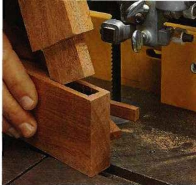
▲ Check Fit in Mortise. Test the tenon fit throughout the process to find the best setup for the fence and stop block. Plane or sand off saw marks for final fit.
