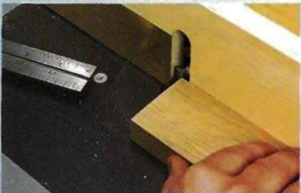
▲ Set the Bit Height. Once the fence is in position, the next step is to set the height of the bit. To do this, you can use a workpiece as a set-up gauge. Set the bit about \frac{1}{8} " above the thickness of the workpiece.
