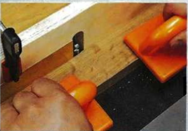
▲ Jointing the Edge. After jointing the first few inches, position your left hand to hold the workpiece firmly against the "outfeed" side of the fence. Padded push blocks provide a firm grip on the workpiece.
