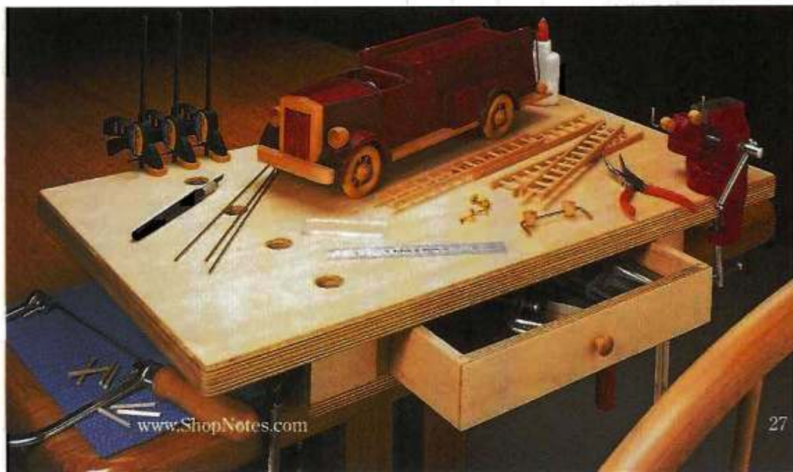
◀ Removeable Top. The top of hobby chest can be removed and used separately.
