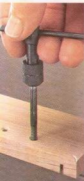
▲ Tapping the Holes. Cutting threads into the holes will hold the machine screws in place.
