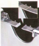
▲ Check Fit. After cleaning the ends of the blade, place them in the brazing jig and check the fit.
