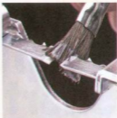
◀ Apply Flux. Using a small brush, apply flux to the mating surfaces of the joint.
