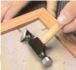
▲ In a Tight Spot. The triangular face of this hammer swivels to make it easy to drive into a corner.
