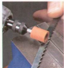
▲ Grind the Joint Smooth. A rotary tool is ideal for removing the excess solder and grinding both sides of the joint smooth.
