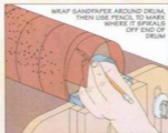
▲ Mark the Strip. At the opposite end of the drum, mark where the strip goes off the end of the drum. Then trim along the line.
