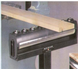
◀ Ramp & Roller. This stand acts as both a bearing stand and a roller stand with just a flip of the top assembly.
