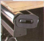
▲ Roller. Flip the bearings down to expose the roller. The bearing assembly acts as a ramp for the workpiece.
