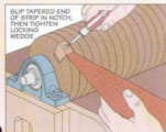
▲ Starting the Strip. After tapering one end of the sanding strip, lock it in place with the wedge and wrap it around the drum.
