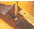
▲ A Turn of the Screw. A very fine turn of the adjustment screws is all it takes to raise or lower the blade.
