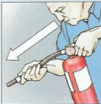
▲ A - Aim. For the best effect, aim the nozzle of the extinguisher at the base of the fire, not at the top of the flames.
