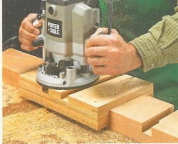
DOG HOLE JIG (TOP VIEW)
