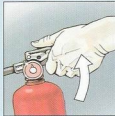
▲ S - Squeeze. Squeeze the lever handles together to allow the propellant to spray the dry chemical onto the fire.
