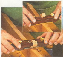
▲ Push or Pull — Always Downhill. The spokeshave can be pushed away from your body, as in the inset photo, or pulled toward it (main photo). But the key is to always cut with the grain or "downhill."
