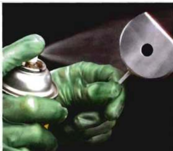
▲ Protect the Shine. A piece of threaded rod and a stop nut make a great handle when spraying lacquer on the fence of the marking gauge.
