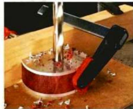
▲ Drill Slowly. To keep the fence from catching on the bit, clamp it to an auxiliary fence and use a slow bit speed.
