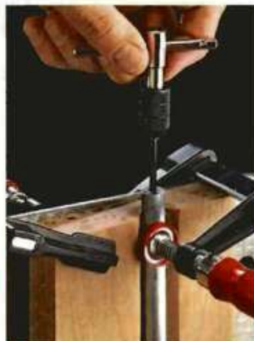
▲ Tapping Threads. After drilling the hole, leave the beam clamped in the V-block for tapping threads.
