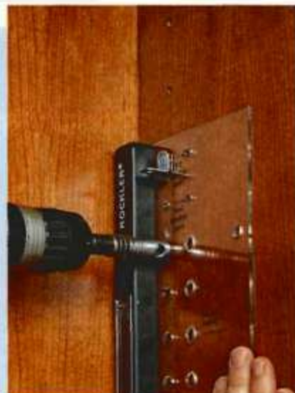
▲ Continuous Drilling. Slip a shelf pin in the indexing hole to keep drilling down the workpiece.
