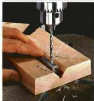
▲ Cutting Pin Hole. Rotate the drill press table square to the bit and drill the hole for the cutting pin.
