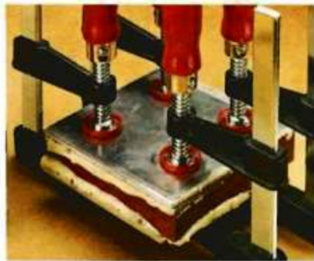
▲ Aluminum Sandwich. Use plenty of clamps and polyurethane glue to join the aluminum faces to the hardwood core.
