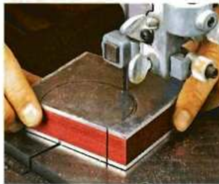
▲ Cut to Shape. A band saw with an ordinary 3/16"-wide blade makes cutting the fence to shape a breeze.
