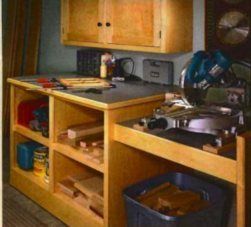
Miter Saw Workcenter
