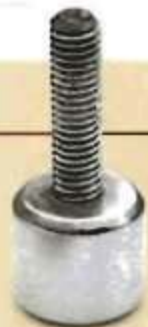
▲ Matching Knobs. The knobs are made just like the beam. Then a threaded stud is glued in place.
