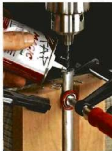
▲ Cutting Oil. A light cutting oil helps cool the bit and remove debris while drilling.
