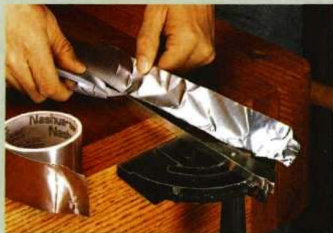
▲ Michael Dingas of Warner Robins, GA, uses metal foil tape used for furnace duct work and repair to tighten the fit of the miter gauge on his table saw. He applies the tape to the edge of a clean miter gauge bar and trims it with a knife.
