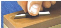
▲ Flatten & Hone. The first step in sharpening the blade of a circle cutter is to flatten the back (left photo). Once that's
