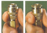
▲ Stay Connected. Some couplers (left) can disconnect if you catch the edge of the sleeve. A drag ring (right) or raised edge prevents this.
