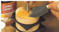
▲ One Layer at a Time. Next, build up the assembly by alternating the rubber gaskets with the MDF disks and gluing them together with contact cement.
