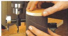
▲ Size the Disks. The first step in building a sanding drum assembly is to use a circle cutter to size the MDF disks so they just slip inside the sanding sleeve.
