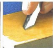
complete, you can hone the bevel. I find it works best to do this by holding it flat against the stone and drawing it back (right photo).
