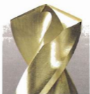
▲ Split Point. The tip is split at the center. This makes starting the hole easier and keeps the bit from wandering as drilling begins.
