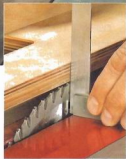
▲ Flush with the Blade. A square can take some of the guesswork out of adjusting the fence.
