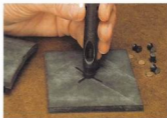
▲ The Gaskets are Next. After cutting squares of rubber to size, create a hole for the drive shaft with a hollow steel punch.
